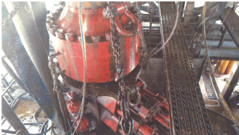
Figure 1: Winch System attached to BOP Stack
