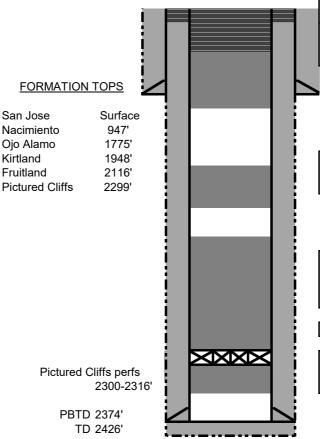
7-11-2022: Top off: Cut off WH, TOC; 4 1/2" csg at 75', annulus at 25'. Install P&A marker, top off with 18 sx.
