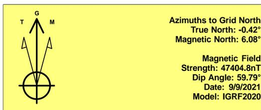
To convert a Magnetic Direction to a Grid Direction, Add 6.08°
