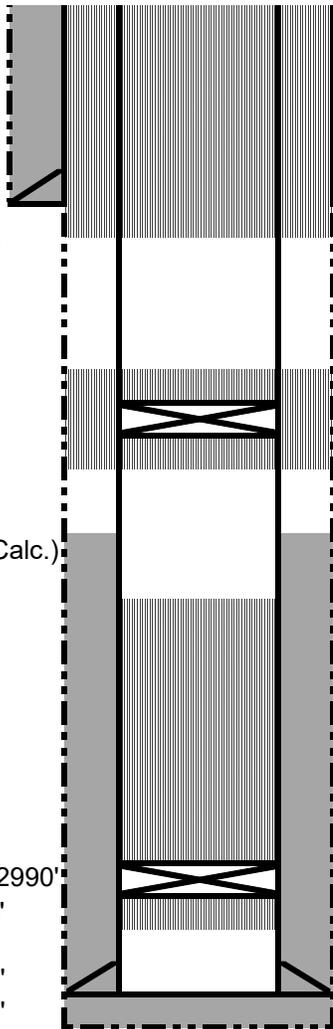
Plug 4 (Surface shoe and surface plug): Perf holes at 144'. Tie onto 4-1/2" casing and mix and pump sufficient volume to bring TOC to surface, inside and outside.
