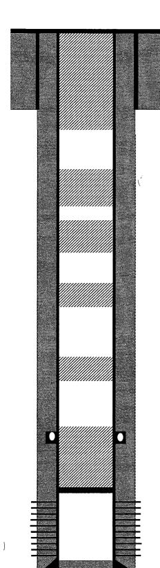
8-5/8" J-55 24# casing @ 201'. Cemented with 135 sks, 159 cf Class B w/ 2% CaCl2. Circulated cement to surface. Hóle size: 12-1/4
