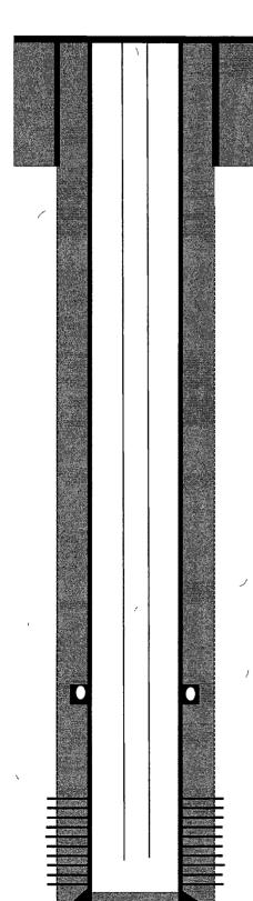
8-5/8" J-55 24# casing @ 201'. Cemented with 135 sks, 159 cf Class B w/ 2% CaCl2. Circulated cement to surface. Hole size: 12-1/4
