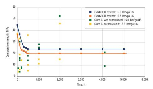
Compressive strength evolution of portland cement and EverCRETE system samples with time in wet supercritical  $CO_2$  fluid and in  $CO_2$  saturated in water at 194 degF [90 degC] under 28 MPa of pressure. After 6 months in  $CO_2$ -saturated water, the compressive strength of portland cement is not measurable because most of the samples are highly deteriorated. The stability of the EverCRETE system minimizes the degradation potential of the long-term barrier.
