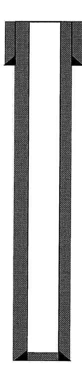
8-5/8", 24# J-55 Casing set @ 132.5' RKB Cemented w/ 200 sks Class B cement w/ 2% Calcium and ¼#/sk CF Circulated 6 bbl cement to surface
