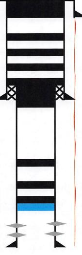
Plug 8 P&S 420 feet - Surface 420 foot plug 110 Sacks of Type III Cement
