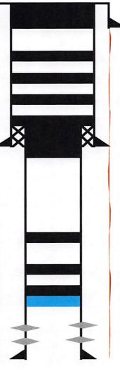
Plug 8 420 feet - Surface 420 foot plug 110 Sacks of Type III Cement
