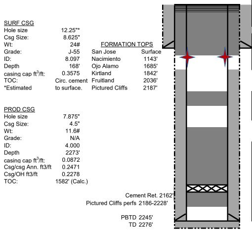
8-26-2022: Cut off WH. TOC at surface. Install P&A marker. Top off with 22 sx.
