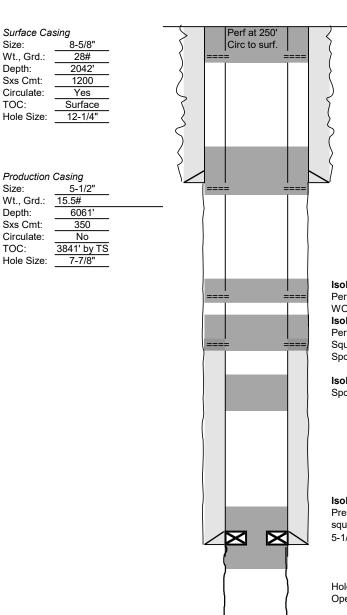
**Isolate Salt, Rustler, 8-5/8" shoe** Perforate at 2100' Squeeze from 2100' to 1600'
