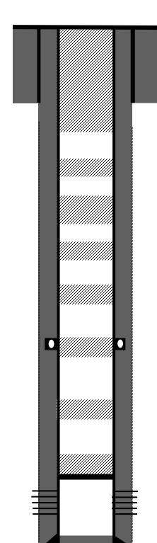
8-5/8" 24# casing @ 312'. Cemented with 211 sks, Class B cement w/ 2% CaCl2. Circulated cement to surface. Hole size: 12-1/4
