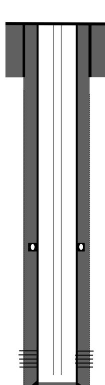
8-5/8" 24# casing @ 312'. Cemented with 211 sks, Class B cement w/ 2% CaCl2. Circulated cement to surface. Hole size: 12-1/4
