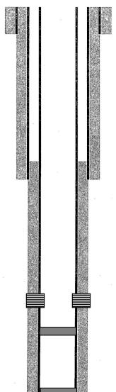
17-1/2" hole @ 855' 13-3/8" csg @ 855' w/ 725sx-TOC-Surf-Circ
