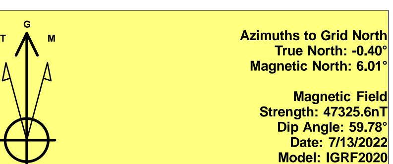
To convert a Magnetic Direction to a Grid Direction, Add 6.01° To convert a Magnetic Direction to a True Direction, Add 6.41° East To convert a True Direction to a Grid Direction, Subtract 0.40°
