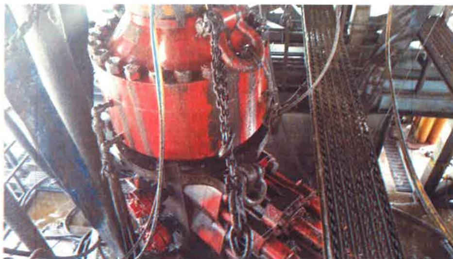
Figure 1: Winch System attached to BOP Stack
