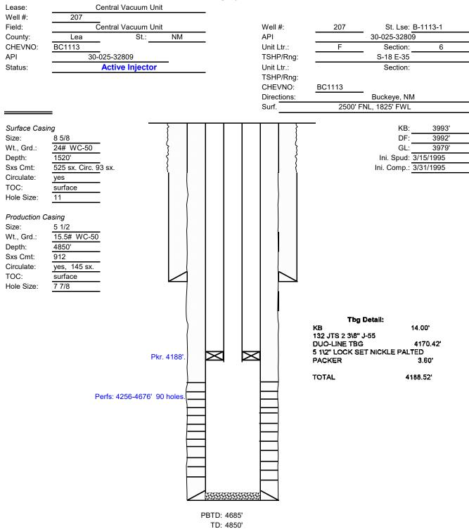
12/12/2022: PHW Wireline: RIH w/1.250" tool string with sample bailer tagged at 4299', recovered sample. (got stuck kept jarring for 20 minutes and was able to pull free. )
