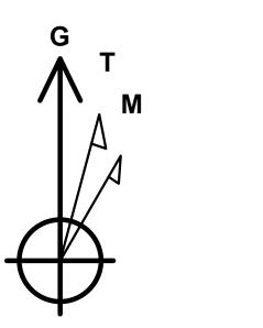
Azimuths to Grid North True North: 0.04° Magnetic North: 6.82°
