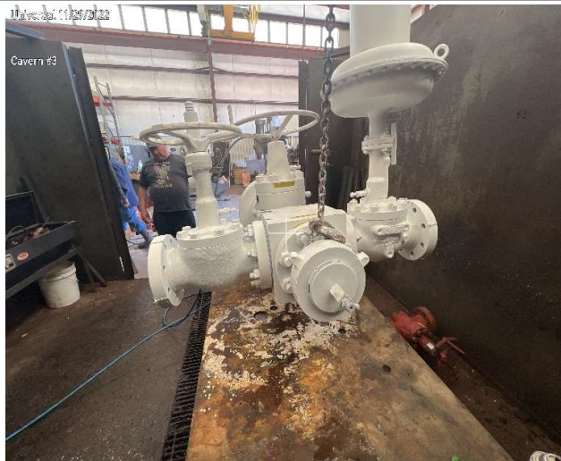
Well head upper section and job stamp on body
