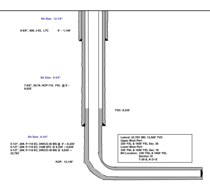
961' FSL 2245' FEL Section 30 T-26-S, R-31-E Proposed Wellbore Design B KB: 3,158' GL: 3,133'
