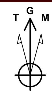
**Azimuths to Grid North** True North: -0.37° Magnetic North: 5.95°
