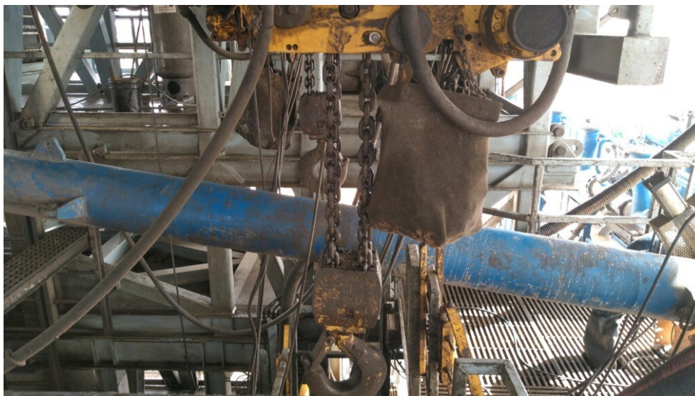
Figure 2: BOP Winch System
