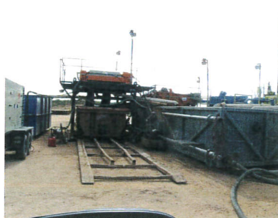
Above: Centrifugal Closed Loop System
