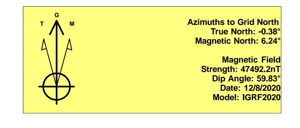
To convert a Magnetic Direction to a Grid Direction, Add 6.24° To convert a Magnetic Direction to a True Direction, Add 6.62° East To convert a True Direction to a Grid Direction, Subtract 0.38°
