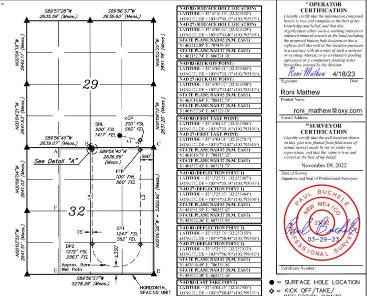
LINE TABLE LINE DIRECTION LENGTH L1 S76°55'37"F 879.95 S00°07'46"E L2 400.00 L3 S00°05'04"E 3936.00 L4 N00°03'27"W 3910.72 L5 N00°06'28"W 90.00'
