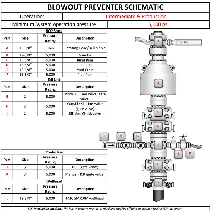
The installed BOP equipment meets at least the minimum requirements (rating, type, size, configuration) as shown on this schematic. Components may be substituted for equivalent equipment rated to higher pressures. Additional components may be put into place as long as they meet or exceed the minimum pressure rating of the system.
