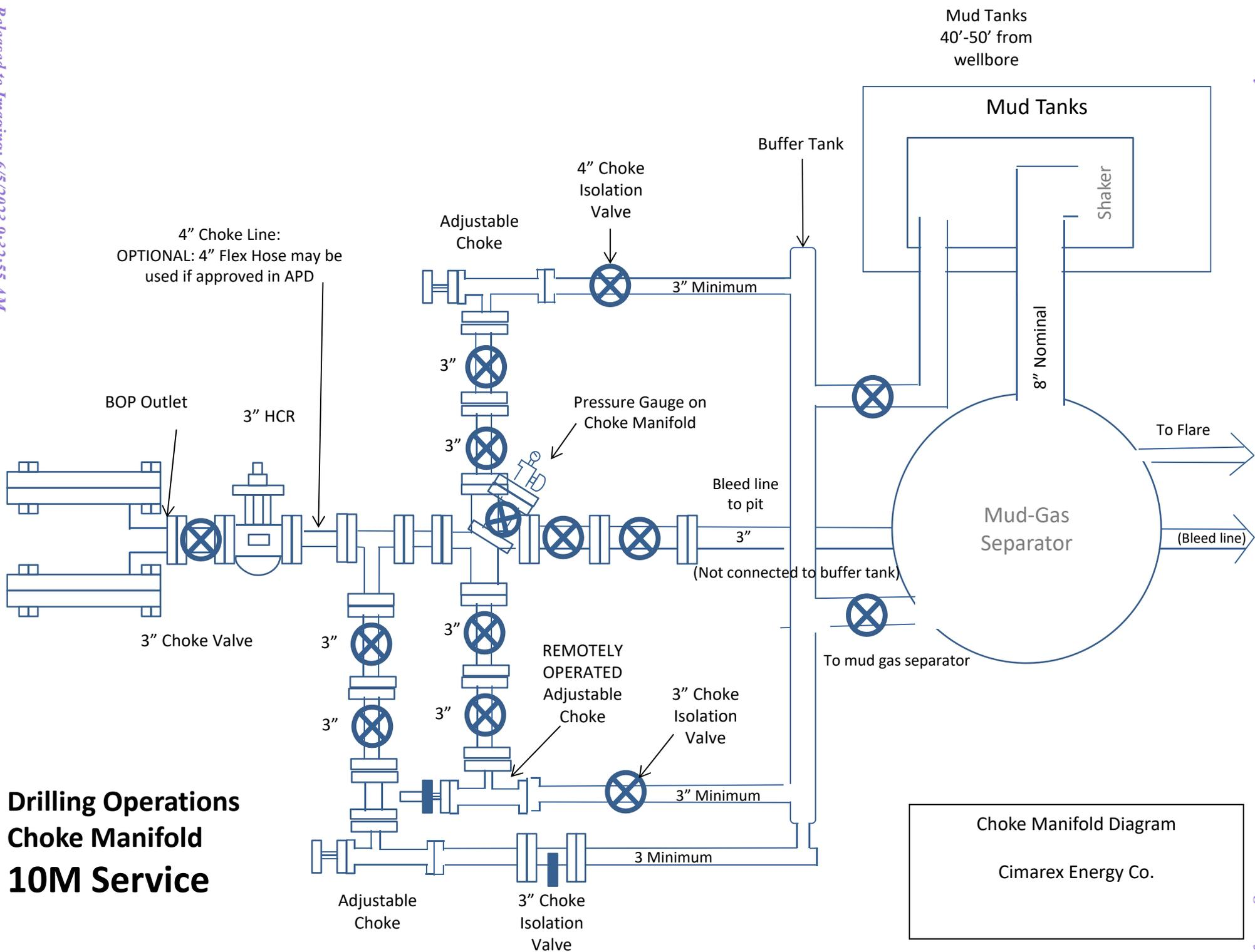
Choke Manifold Diagram
