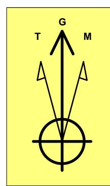
**Azimuths to Grid North** True North: -0.35° Magnetic North: 6.26°
