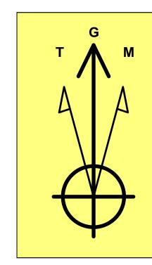
**Azimuths to Grid North** True North: -0.35° Magnetic North: 6.13° **Magnetic Field** Strength: 47395.0nT Dip Angle: 59.88° Date: 7/1/2022
