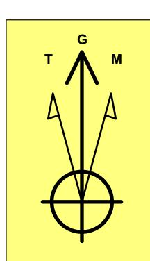
**Azimuths to Grid North** True North: -0.35° Magnetic North: 6.26°
