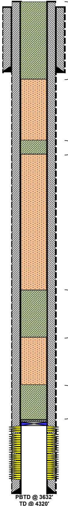
4. PUH & spot / fill up with 50 sx Class "C" cmt from 487' to surf. (Surf Shoe, Water Board, & Surf Plug)
