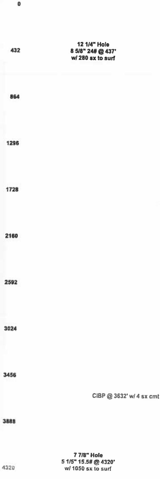
4. PUH & spot / fill up with 50 sx Class "C" cmt from 487' to surf. (Surf Shoe, Water Board, & Surf Plug)
