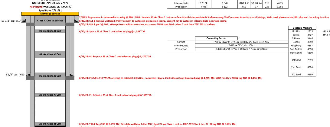
6/15/23: RIH & set CIBP @ 8,800' WLM; Load casing & test to 500 psi for 30 minutes, good test.
