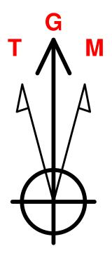
Azimuths to Grid North True North: -0.18° Magnetic North: 6.44°
