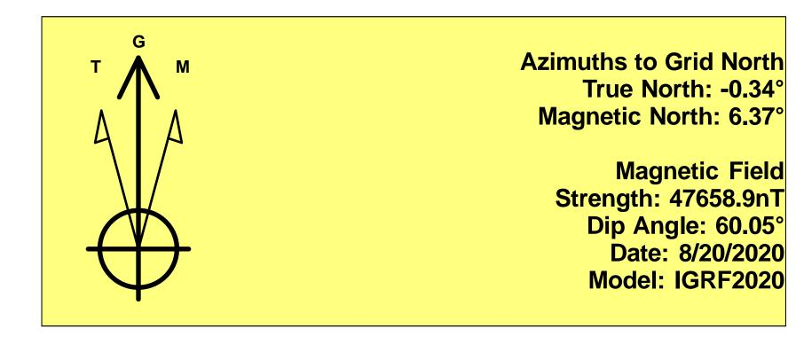
To convert a Magnetic Direction to a Grid Direction, Add 6.37° To convert a Magnetic Direction to a True Direction, Add 6.71° East To convert a True Direction to a Grid Direction, Subtract 0.34°
