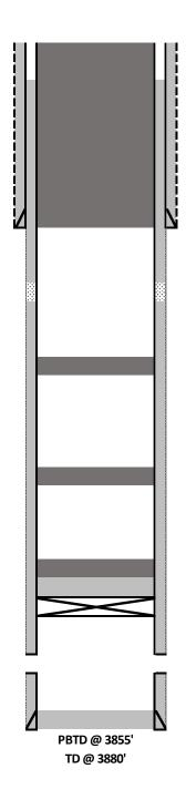
8-5/8" CSG @ 306' Perf & Sqz. 140 sks class C cement 356' - surface. Tagged @ surface.
