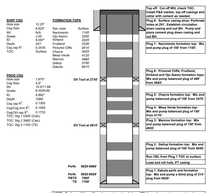
NOTE: Portions of the wellbore have not previously been CBL logged, cement coverage is unknown, a CBL will be run to determine how cement plugs are to be placed. Perforations and cement retainers, if needed, will be placed and cement plugs placed, (inside or inside/outside) in conformance with P&A requirements and COA.
