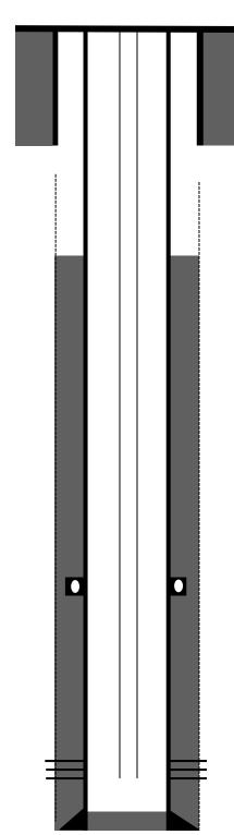
8-5/8" J-55 24# casing @ 236' . Cemented with 125 sks Class B. Circulated cement to surface. Hole size: 12-1/4
