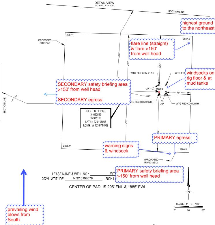
ALL BEARINGS, DISTANCES, AND COORDINATE VALUES CONTAINED HEREON ARE GRID BASED UPON THE NEW MEXICO COORDINATE SYSTEM, EAST ZONE OF THE NORTH AMERICAN DATUM 1983, U.S. SURVEY FEET
