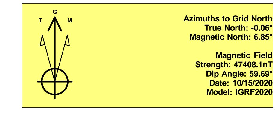
To convert a Magnetic Direction to a Grid Direction, Add 6.85° To convert a Magnetic Direction to a True Direction, Add 6.91° East To convert a True Direction to a Grid Direction, Subtract 0.06°
