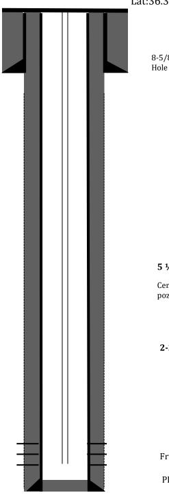
8-5/8" 24# casing @ 132'. Cemented with 95 sks Class B cement. Hole size: 12-1/4". Circulate 7 bbls cement to surface.
