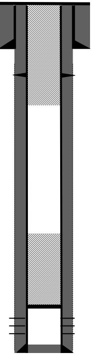
8-5/8" 24# casing @ 132'. Cemented with 95 sks Class B cement. Hole size: 12-1/4". Circulate 7 bbls cement to surface.
