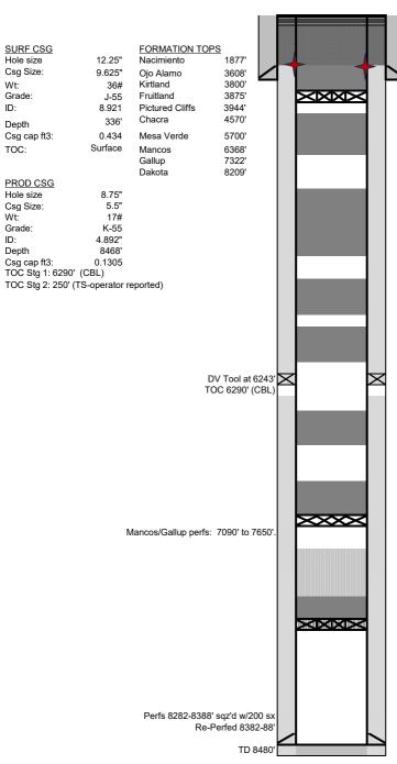
8-31-2023: Cut off WH. TOC, 24' in 9 5/8" casing, 65' in 5 1/2" casing. Install P&A marker. Top off casing and cellar with 40 sx.
