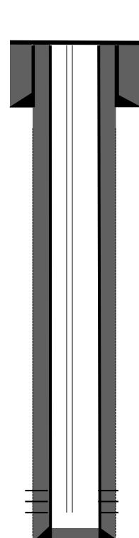
8-5/8" 24# casing @ 140'. Cemented with 135 sks Class B cement. Hole size: 12-1/4". Circulate 7 bbls cement to surface.
