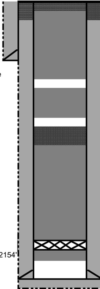
10-9-2023: Top off: Cut off WH. TOC at surface in 4 1/2" casing and 50' in 8 5/8" casing. Install P&A marker. Top off casing and cellar with 30 sx.
