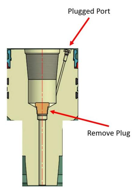
This method would leave two tests that cannot be performed with drill pipe acting as the leak path. Lower pipe rams and blind rams. To test the lower pipe rams we need to open port on top of the test plug and add the inner plug back in. Blind rams would be tested against casing with no test plug installed. Due to no leak path these would be 30 min high/low tests with <10% bleed off.
