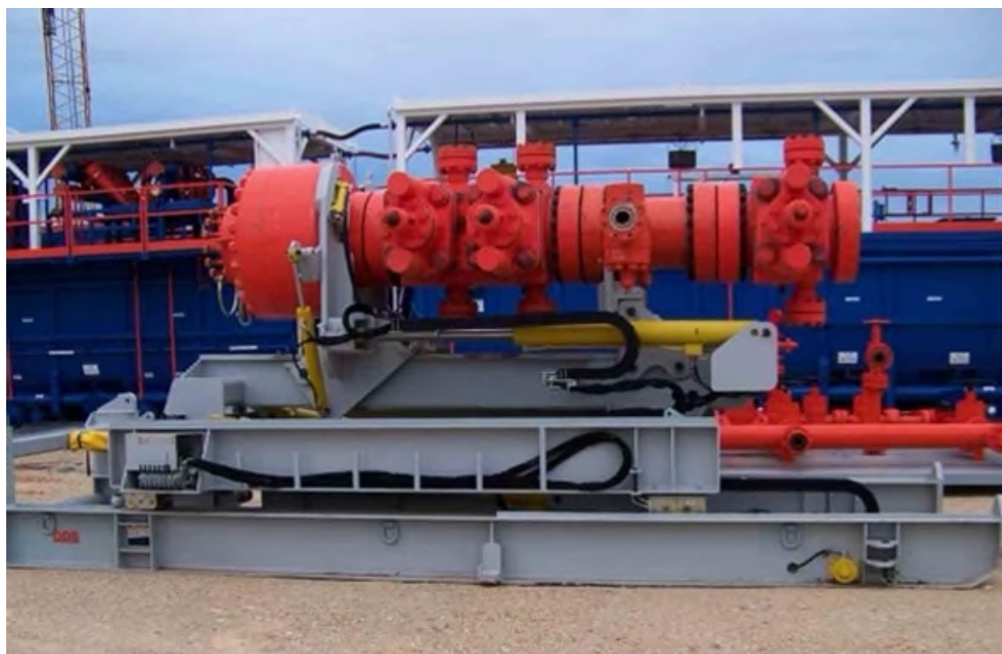
Figure 4. BOP handling system
