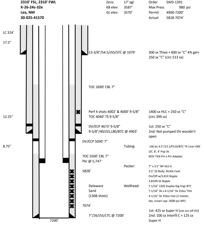
Jul 2015: Went into service. Jan 2019: Repair WO tbg/pkr leak. Dec 2023: Repair WO tbg/pkr leak.
