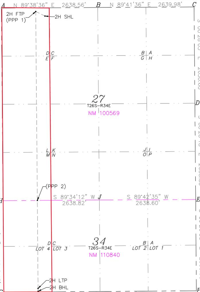
The diagram shows a survey plat for sections 27 and 34. Section 27 is outlined in red and contains well locations 2H FTP (PPP 1), 2H SHL, and 2H LTP. Section 34 contains well location 2H BH. The plat includes bearings and distances for all boundaries, such as N 89°38'36" E 2638.56' and S 89°34'12" W 2638.82'. It also shows the locations of kick-off points, first and last take points, and the bottom of the hole. A grid of corner points A through S is provided for reference.
