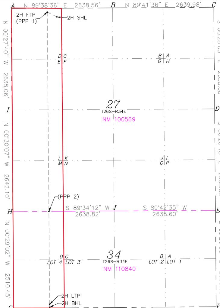
The diagram shows a well location plat for BOLL WEEVIL 27-34 FED COM. It features a central well location (2H FTP) and a bottom hole location (2H SHL). The plat is bounded by sections 27 and 34, and lots 1, 2, 3, and 4. The diagram includes bearings and distances for all boundaries, such as N 89°38'36" E 2638.56' and S 89°34'12" W 2638.82'. It also shows geodetic coordinates for various points (A through J) and the well location (2H LTP, 2H BH).
