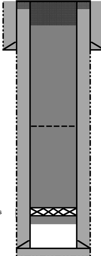
11-22-2023: Cut off WH, TOC in 7" casing at 11'. Install P&A marker. Top off casings and cellar with 20 sx.
