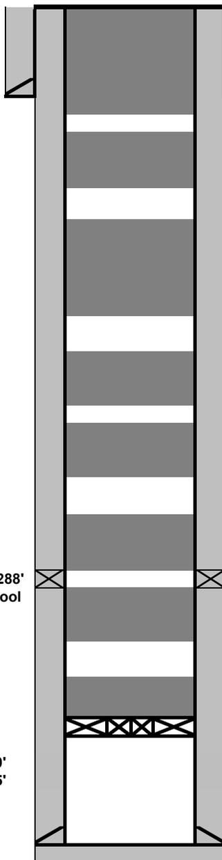
**Plug 8:** Surface casing shoe to surface: Mix and spot balanced plug from 606' to surface. Cut off WH, install P&A marker
