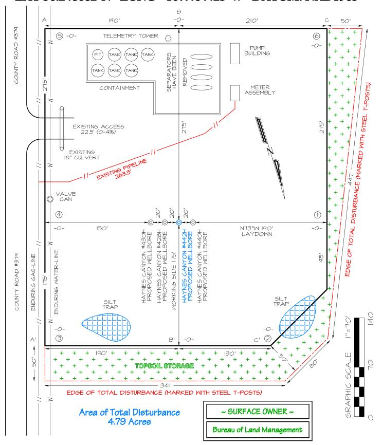
Steel T-Posts have been set to define Edge of Disturbance limits which are 50' offset from edge of wellpad, unless otherwise noted. Some areas have been restricted or omitted as shown hereon.
