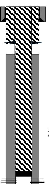
7", 26# Surface Casing Set @ 46'. Cemented w/ 5 sks cement. Hole size 8-3/4"
