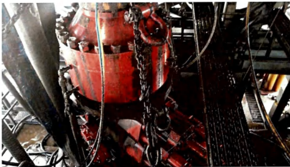
Figure 1: Winch System attached to BOP Stack
